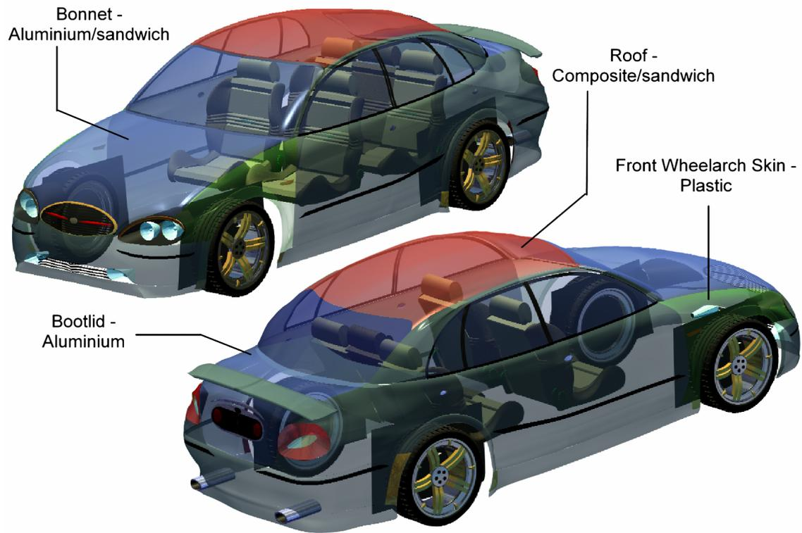
Figure 7. Ford Falcon Conceptual Model A.
