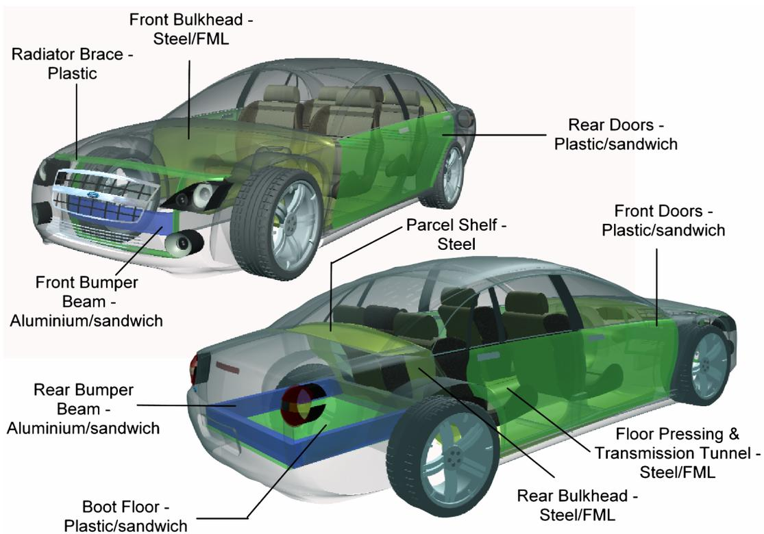
Figure 8. Ford Falcon Conceptual Model B.
