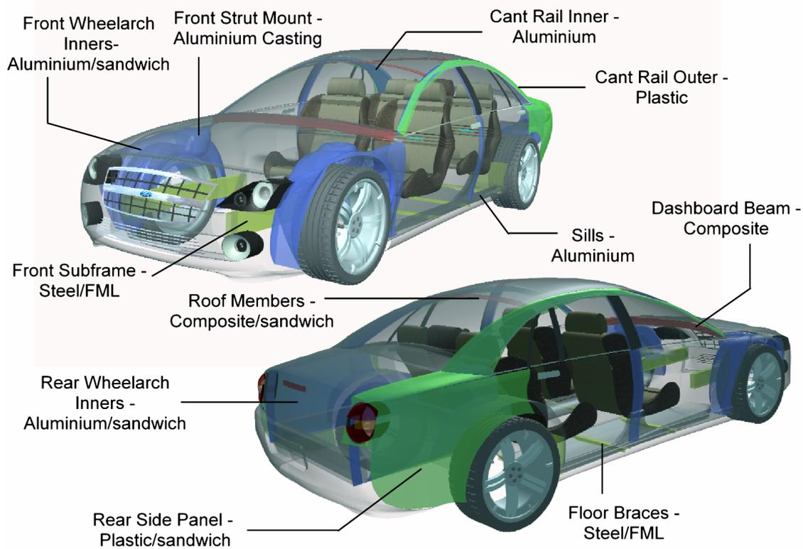
Figure 9. Ford Falcon Conceptual Model C.
