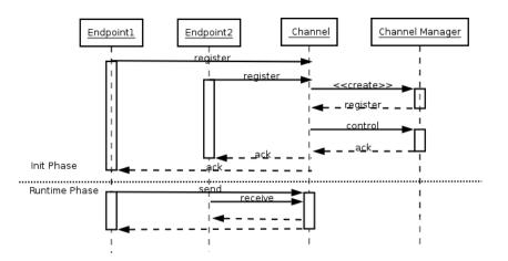
Figure 6. Communication channel and Channel Manager interaction
