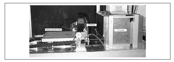
Figure 4: The core parts of the prototype: A substrate held in a substrate holder, which receives the ink as it passes under a printhead and the ink is then hardened on exposure to ultra-violet radiation.
