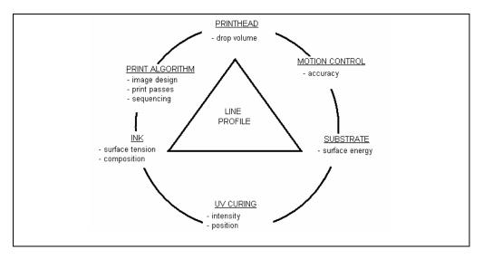
Figure 7: The ink-jet triumvirate expanded to include the secondary subsystems and individualised for line profile.
