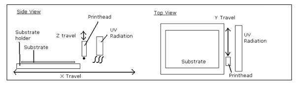
Figure 5: The three axes of motion. As an operator of the machine would see it; the substrate table moves left to right (X axis) passing the substrate under the print-head and the UV radiation. The printhead is able to index, either toward or away from the operator (Y axis), this allows the print-head to cover more of the substrate with more swathes of the image. The distance of the print-head above the substrate is maintained at a safe working distance (Z axis.)
