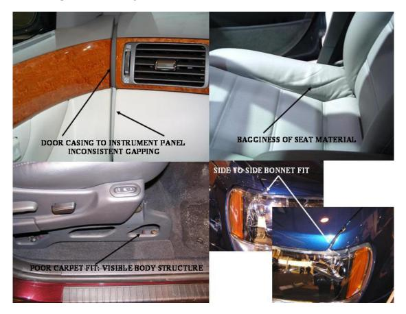
Figure 2: Poor Examples of Craftsmanship Execution
