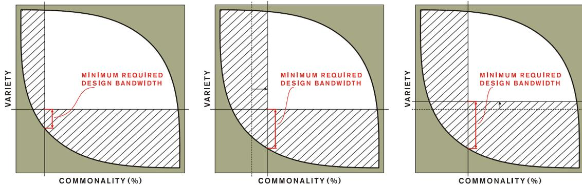
Figure 5. Design bandwidth illustrated in the VC-D space.
