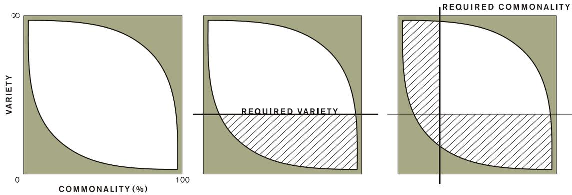
Figure 3. Variety and Commonality – Design (VC-D) space illustrating the effects of the relationship between variety and commonality.
