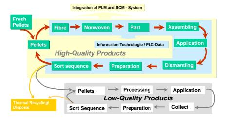
Figure 6. The Controlled Closed Loop Recycling
