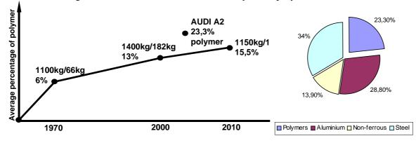
Figure 1. Average percentage of polymer automotive parts [1]
