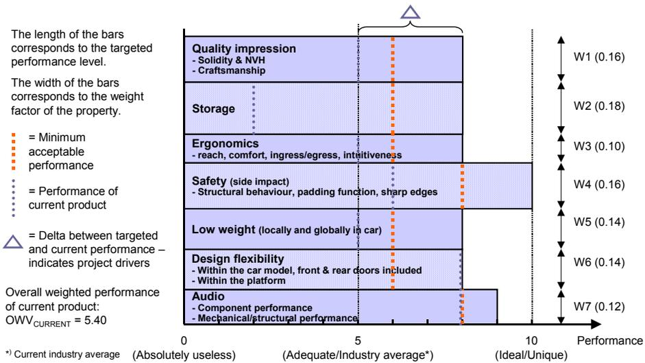
Figure 5. Desired performance profile for the next generation door module.
