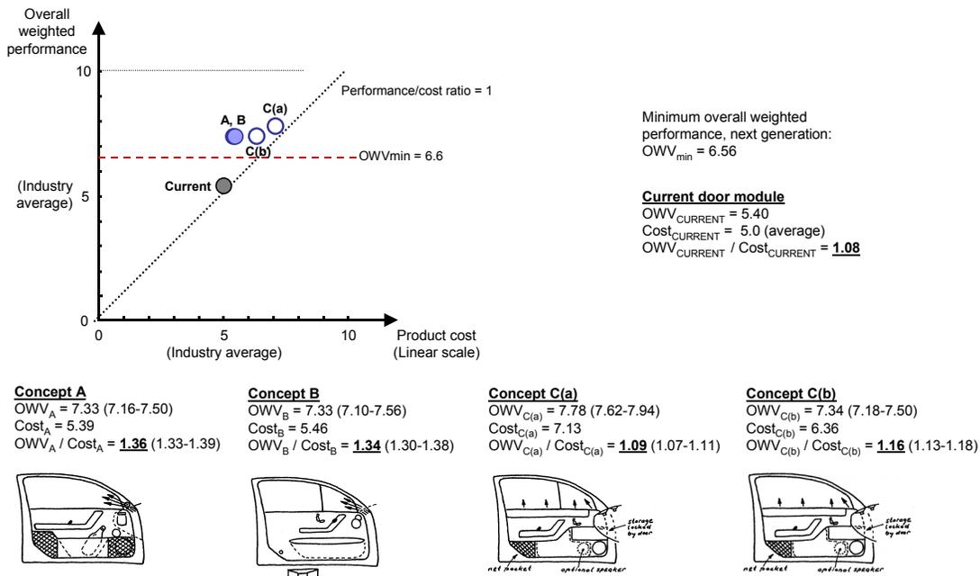
Figure 9. Performance/cost ratio for the four synthesised concepts (indexed cost).
