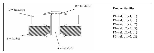
Figure 4. Example of an assembly.
