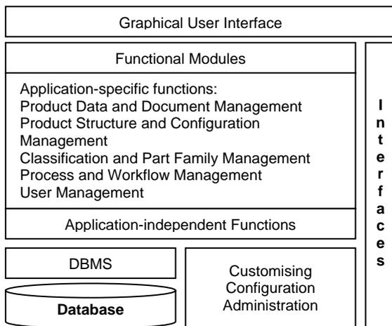
Figure 1. PDM system architecture [1]
