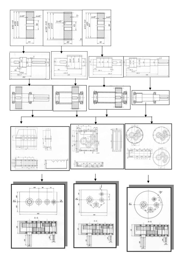
Fig. 5. Scheme of objects of three-stage spur train according principle "from an overall view to the details"
