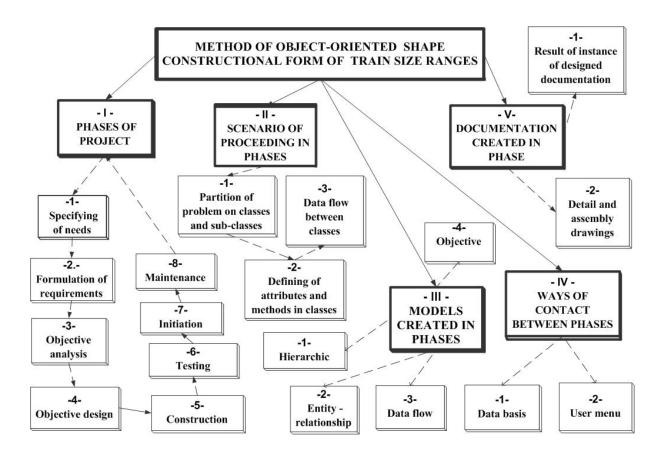
Fig. 3. Elements of design process and output of offered method
