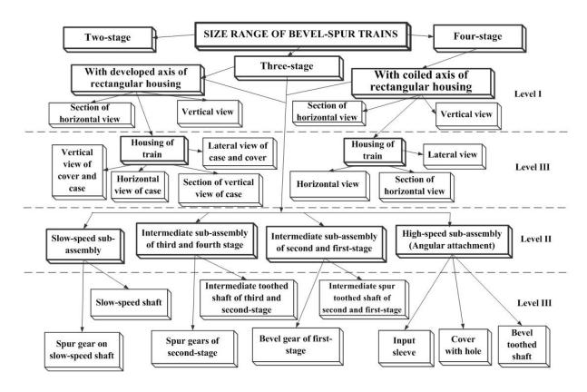
Fig. 4. Scheme of hierarchical model of size ranges of three-stage bevel-spur trains
