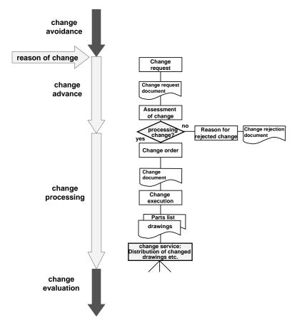
Figure 2. The change process according to DIN 199-4 [DIN 199-4, 1981]
