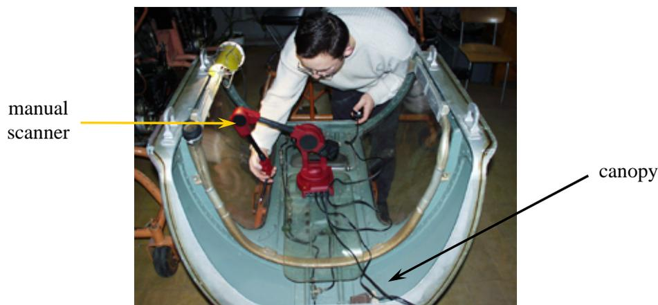
**Figure 1. Measurements of the canopy's shape**
