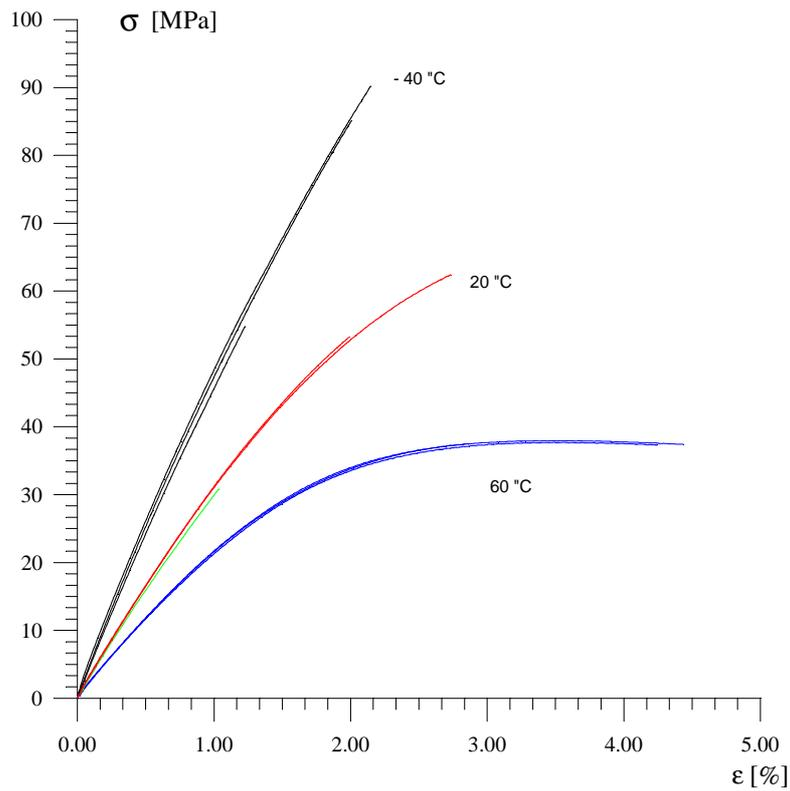
**Figure 3. Results of materials tests**
