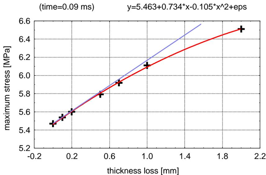
**Figure 7. Maximum material effort (Mises) against changes in glass thickness**
