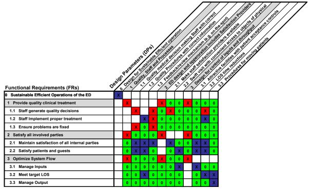
Figure 1. Two Level ED<sup>3</sup> Matrix. All level one FRs and DPs are coupled.
